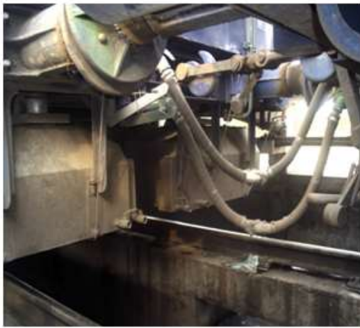
Fitted with four Bio digester tank
