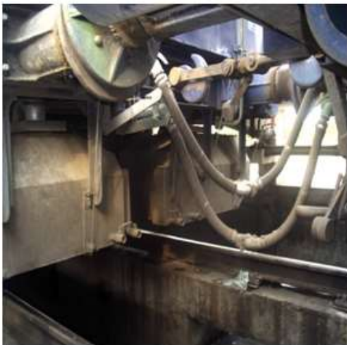
Fitted with four Bio digester tank
